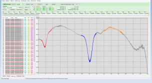
The product will be irradiated with a special developed Halogen lamp. The resulting diffuse reflection (the diffuse reflection contains the necessary information of the constituents) is transmitted via a fibre optic to the spectrometer. The spectrometer split the spectra in 256 support points.
